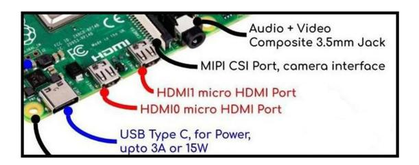
If using an argon one case the HDMI0 will be closest to the edge of the case as shown in picture.
